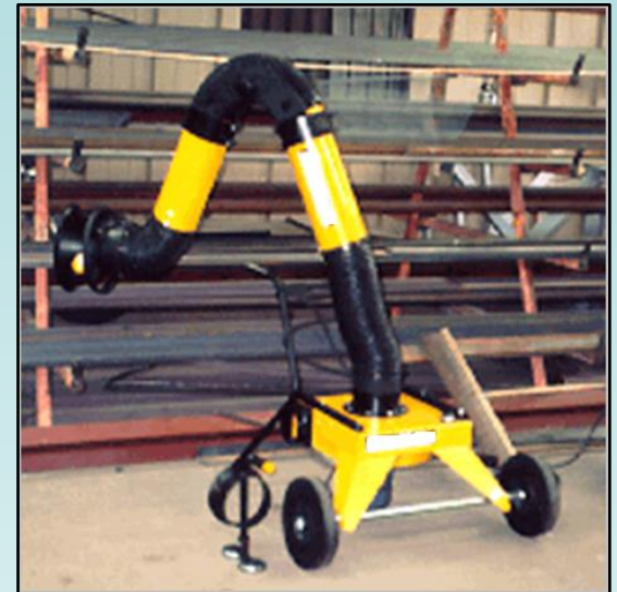
Local Exhaust Ventilation
